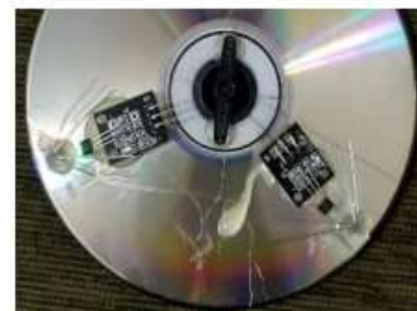
Fig. 3. Hall sensors on the working area of the DT device "Reflex-TH3" (bottom view)
